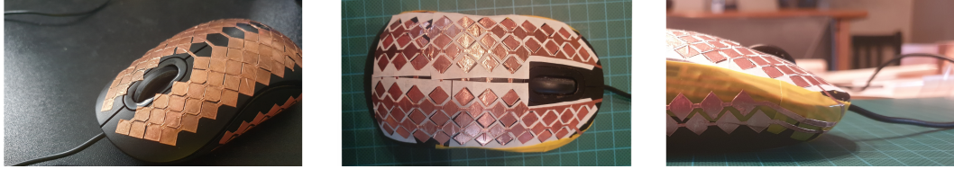
Fig. 1. From left to right: 1. Version 2 of the traces on the mouse. 2. Final version of the traces placed on the mouse with insulation layer. 3. Close up of the direction of the traces in the final version (See also figure 7 in the appendix.
